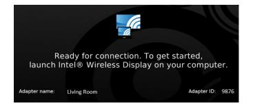
If you do not see this screen, make sure that the TV input is set to the HDMI port where the Push2TV adapter is connected and all cable connections are firmly secured.
